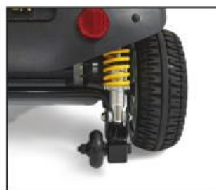
Comfort Spring Suspension Manually adjustable preload on rear suspension!
