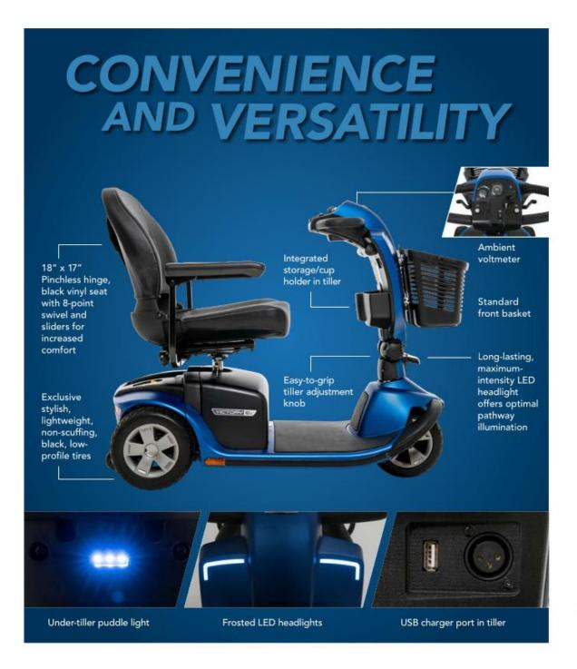
The Victory® 10.2 offers great convenience and versatility with exclusive feather-touch disassembly and a delta tiller with wrap-around handles. Contemporary features such as the integrated storage/cup holder on the tiller ensure ample storage options, while a new under-tiller puddle light offers improved visibility to both the storage area and USB charging port.
