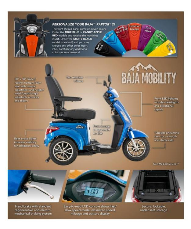
Enjoy fast speed and advanced safety features, all in one sleek package! The Baja™ Raptor 2 cruises up to 14 mph and is equipped with a full LED lighting package and a regenerative braking system.
